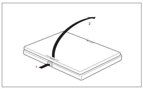
▶ Press the release button (1), and unfold the LCD screen upwards (2).
